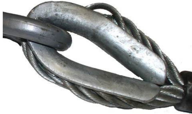
Figure 8. Deformed Thimble and Hook
