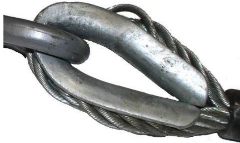
Figure 8. Deformed Thimble and Hook
