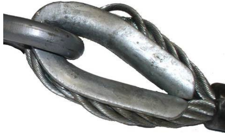
Figure 8. Deformed Thimble and Hook
