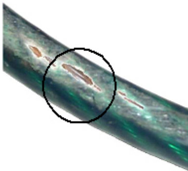
Figure 5. Damaged plastic coated wire rope.
