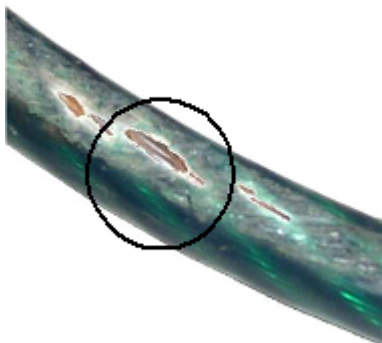
Figure 5. Damaged plastic coated wire rope.
